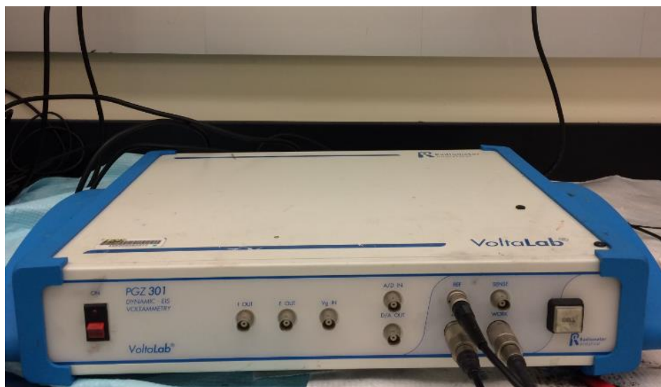
Figure 28 VoltaLab instrument for CV and CA measurements.
